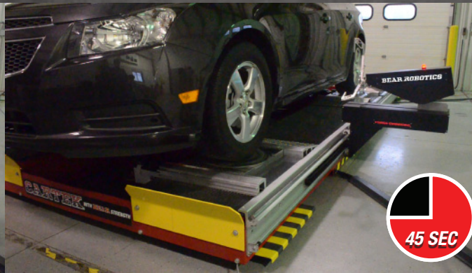
Robots glide across aluminum rail quickly touching rear wheel taking an accurate measurement.
